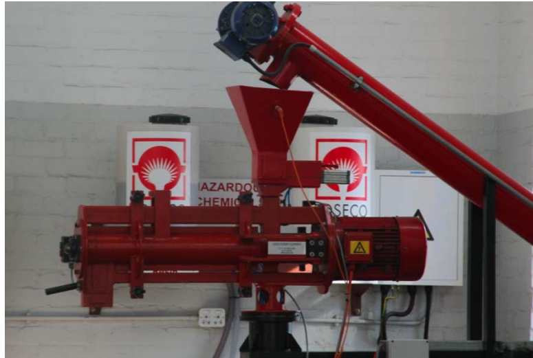
Figure 4.3: Continuous sand mixer installed at the Western Cape Foundry Training Centre.
