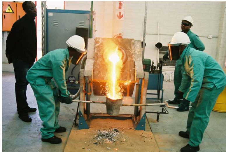
Figure 4.2: Small-scale induction melting furnace for cast iron installed at the Western Cape Foundry Training Centre.
